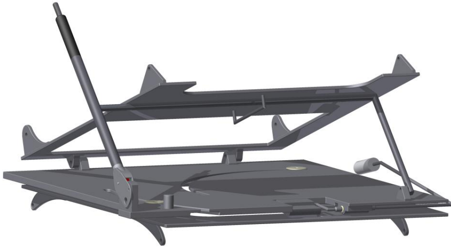
Figure 15. Isometric view of the mechanism with the tilting movement (front-top-left).
