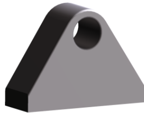
Figure 25. View of the piece where the axle for the tilting lever is inserted.
