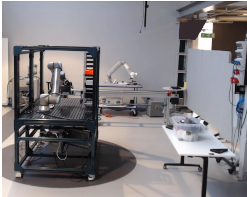
Figure 2: Mock-up assembly station consisting of a battery assembly robot cell, a table, and rearrangeable objects.
