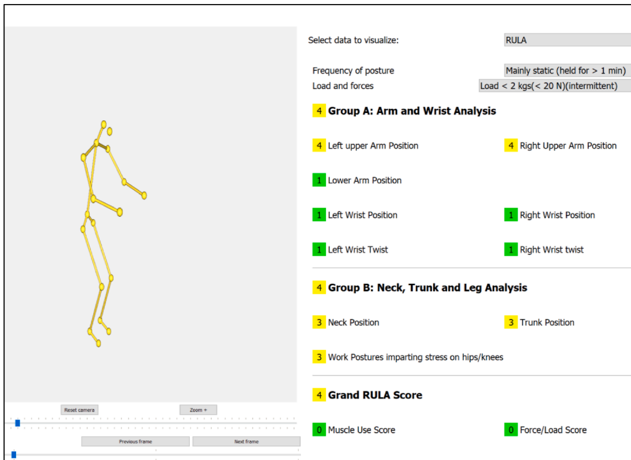
Fig. 5. Manikin and automatic well-being analysis in EPP – Example of RULA analysis made in EPP with postural data from the DHM tool.
