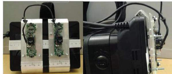
Fig. 5: Video-based prototype in form of a modified Oculus Rift.
