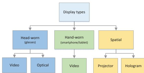
Fig. 4. Different types of displays and hardware used for augmented reality.
