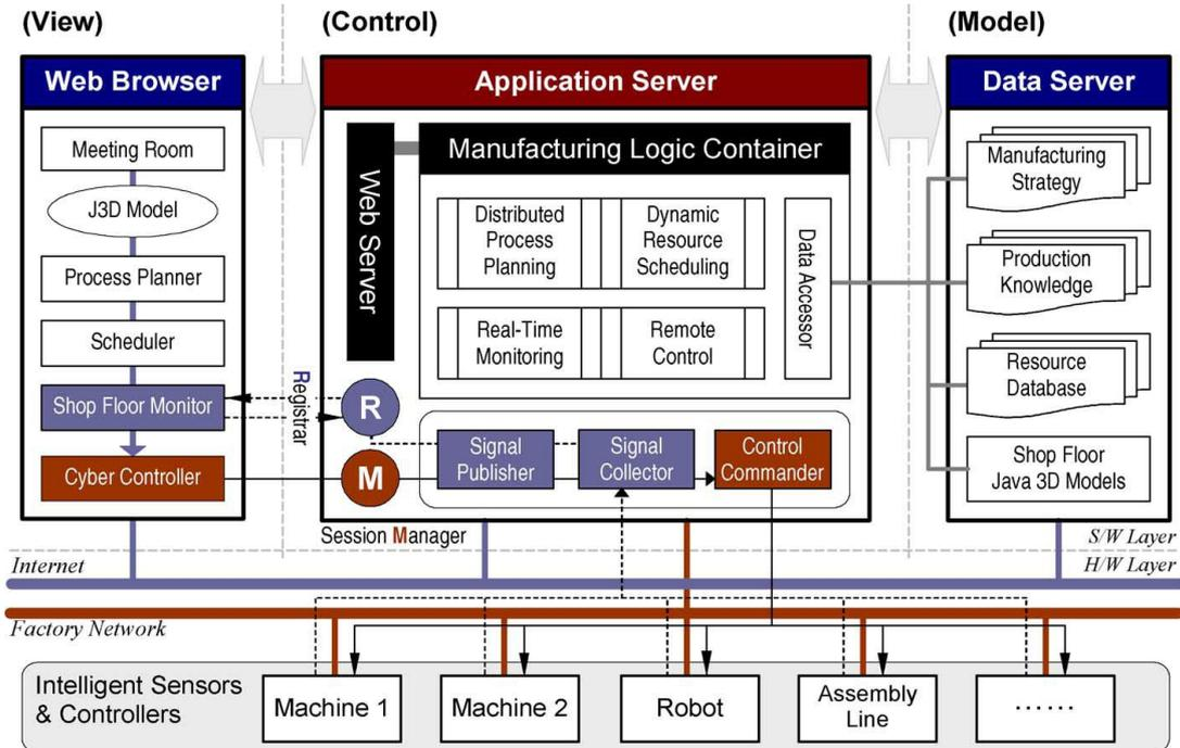
Figure 2. Design of framework for *Wise-ShopFloor*
