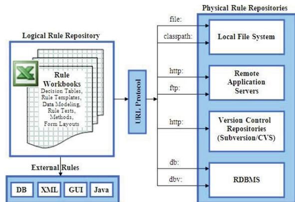
Fig. 3. Architecture of OpenRules (from <http://openrules.com/>).
