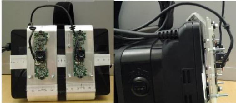
**Figure 1.** Cameras mounted on Oculus Rift.
