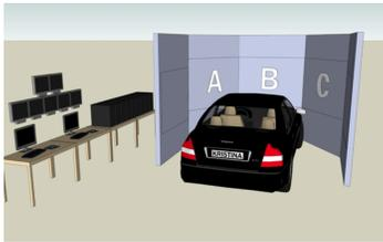
**Figure 3:** Schematic of the vehicle simulator at the University of Skövde: a complete, real car is surrounded by seven screens (two screens behind the vehicle – visible in rear-view mirrors – are not shown on the schematic) on which the environment is projected, creating an immersive experience.
