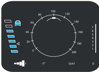
**Figure 2:** The UI element used on the dashboard to indicate vehicle confidence in its automation. Figure adapted from [5].
