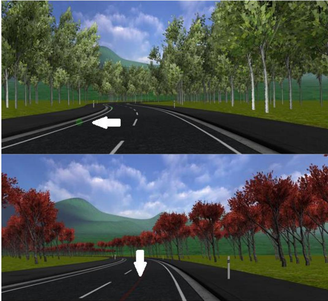
**Figure 8** A Reverse curve and the use of points near tangent point and a Compound curve with the drawn trajectory as appeared in the actual prototype, highlighted by a white arrow for clarity.
