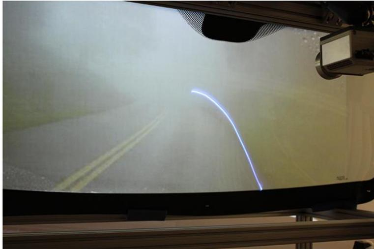
**Figure 12** The use of a Head-Up Display in order to highlight the side of the road in presence of fog. HUD system photo: General Motors. Taken from <http://www.wired.com/2010/03/gm-next-gen-heads-up-display/>
