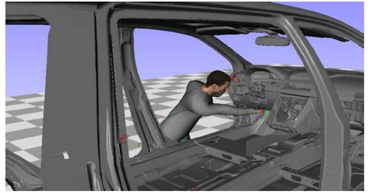
Figure 3. Manikin assembling a part in a narrow area.
