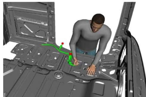
Figure 1. Manikin assembling cables with clips.
