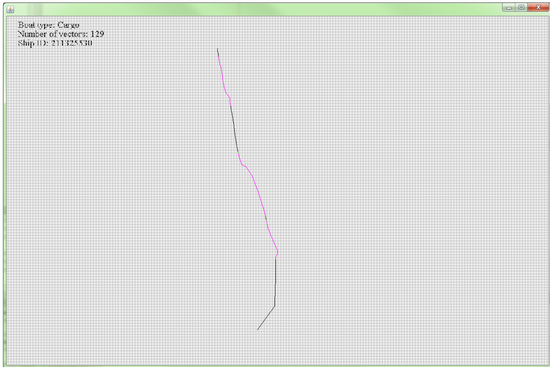
4-14 Course for a cargo ship with marked turns. The purple areas denote a turn, and the green and red denote the start and end of one respectively.
