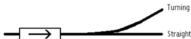
**Figure 10:** A switch is in one of two states: straight or turning.
