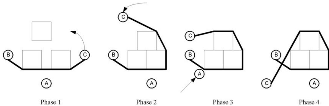
Figure 2 - Three robots tying a rope around three boxes, redrawn from Donald *et al.* (2000).
