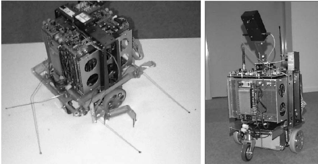
**Figure 11 - Cleaning robots used by Jung and Zelinsky (2000), on the left we see the brush robot and on the right the vacuum robot. With courtesy of Jung.**
