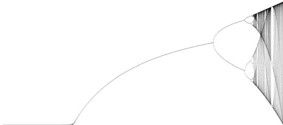
Figure 39: The attractors of f_a as a function of a . from a = 0.0 to a = 3.0 the attractor is a fixed point. At a = 3.0 a bifurcation occurs when the attractor becomes periodic. At higher values of a the attractor sometimes is strange, or chaotic.
