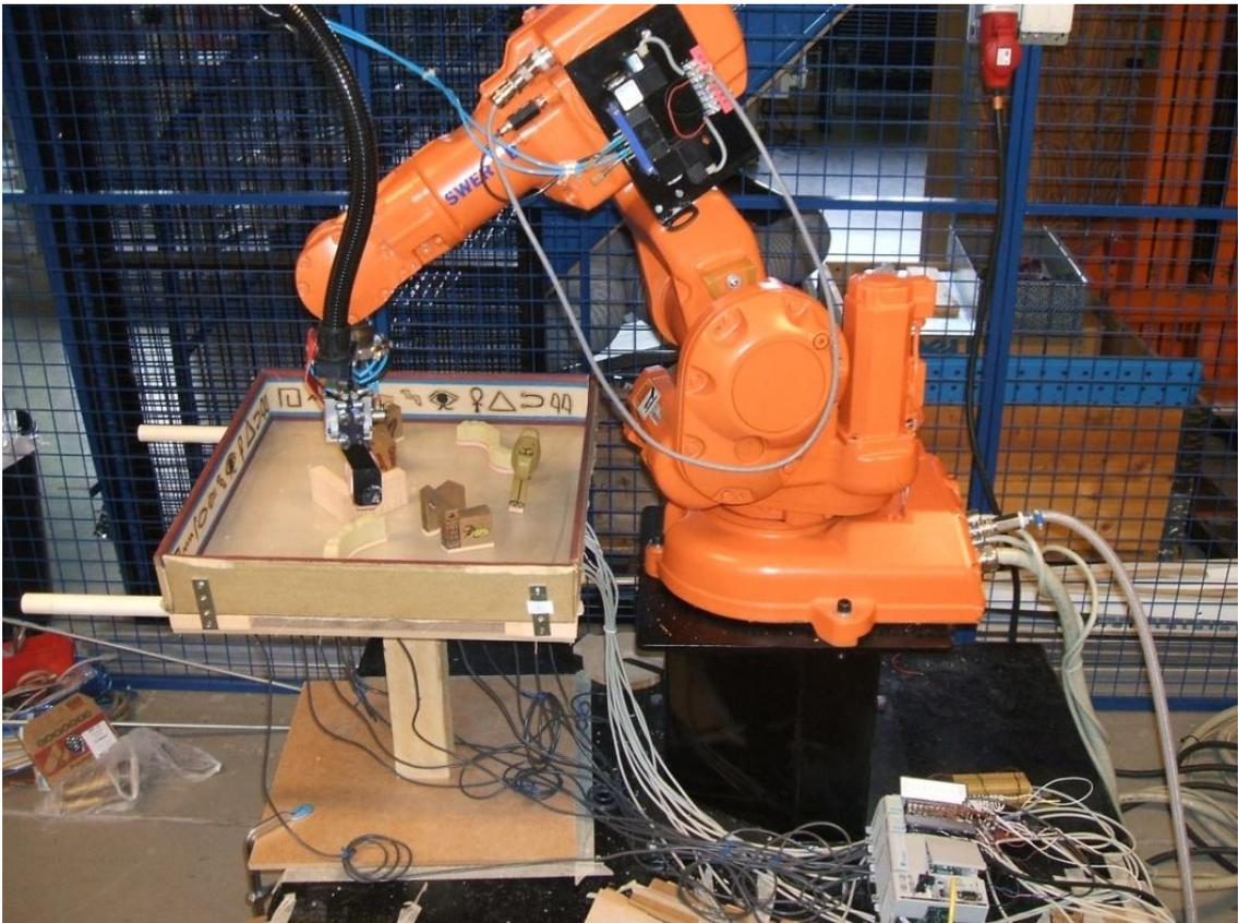
Figure 44 The final board with the robot after prototyping phase.
