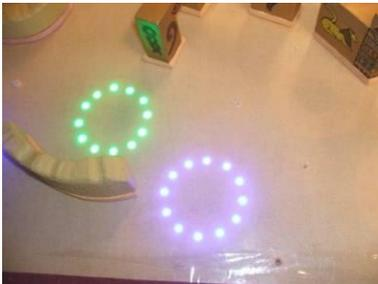
Figure 41 Ring of diodes shining through the fabric and the plexiglass board.
