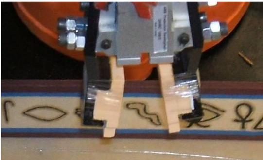
**Figure 49 Rebuilt gripper accessory**
