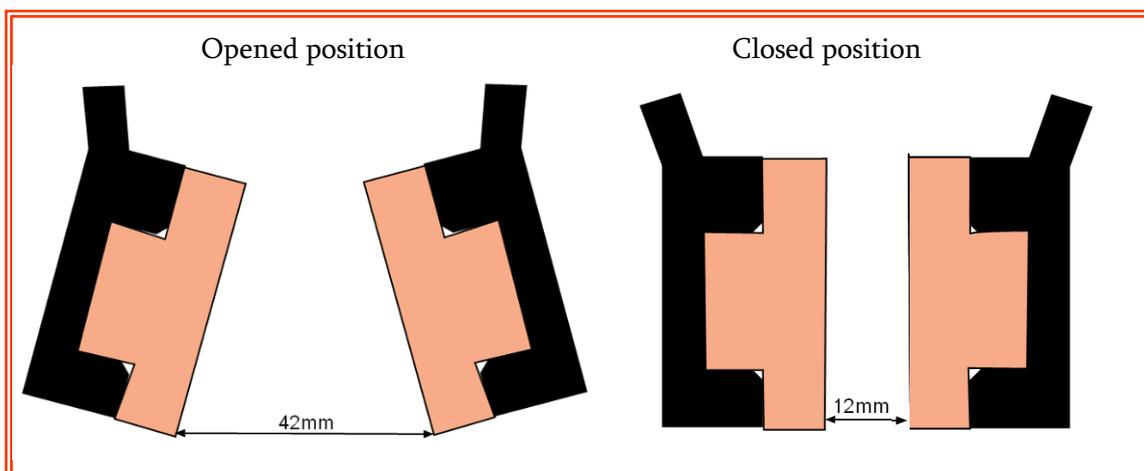
Figure 55 The gripper range
