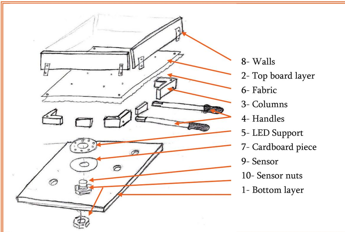
Figure 36 Explosion view of the board components
