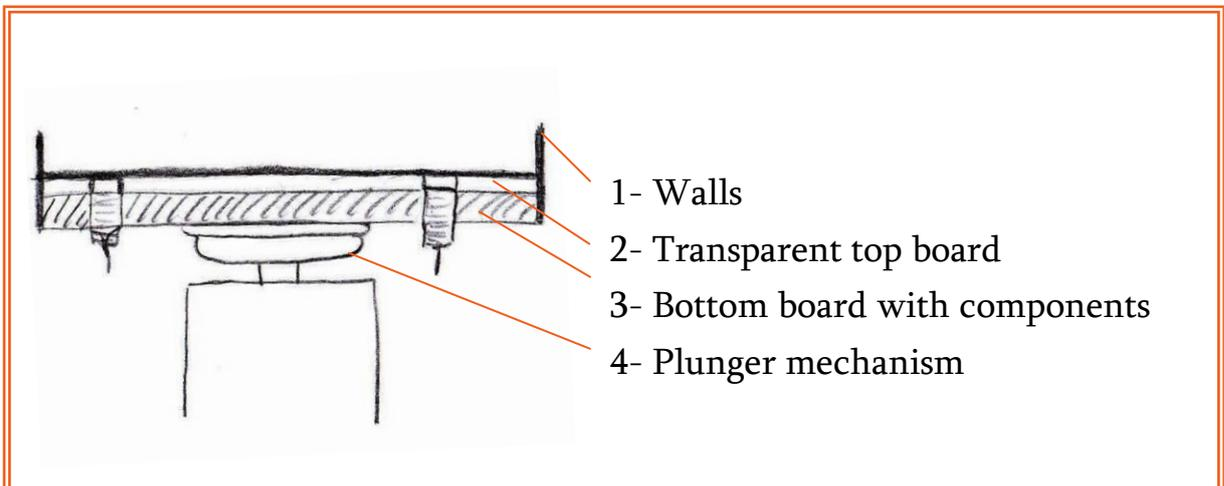
Figure 25 Sketch of the plunger movement
