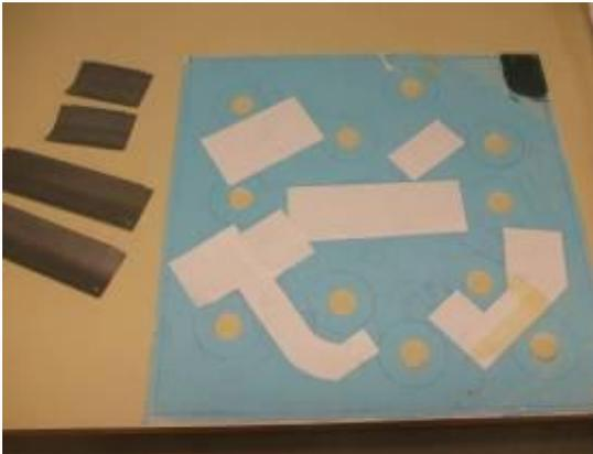
**Figure 27** Disposition of the metal layer on the board for the magnet attachment
