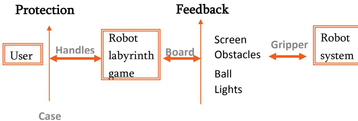
Figure 6 Diagram of game components and functions
