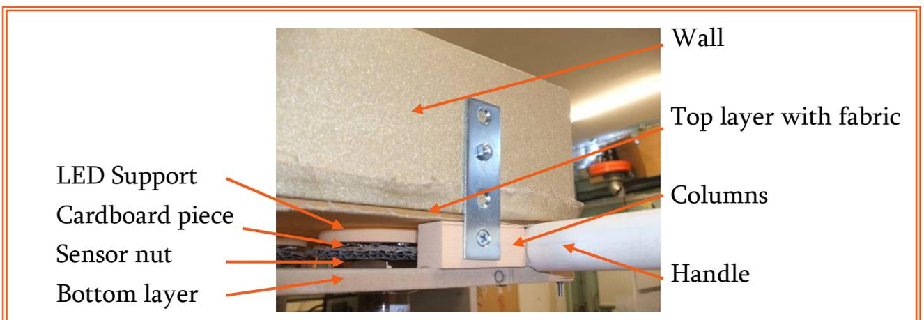
**Figure 42 Detailed components of the assembled board corner**
