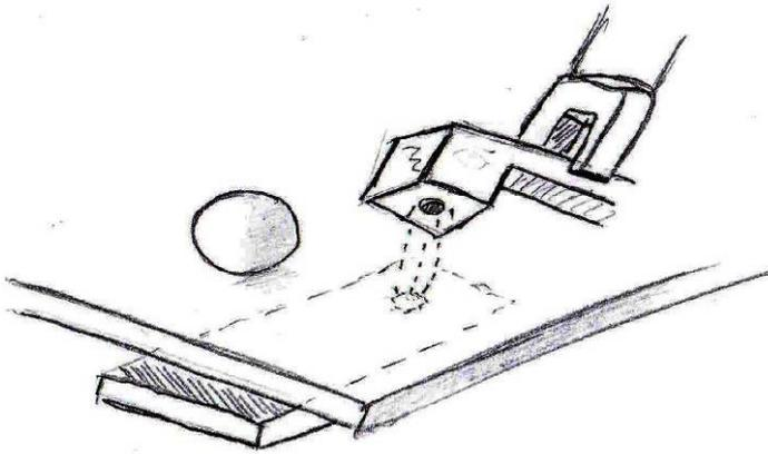
Figure 18 Sketch of the magnet obstacle attachment
