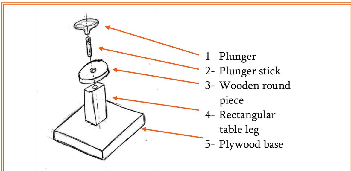
Figure 34 Game board and mechanism assembly explosion
