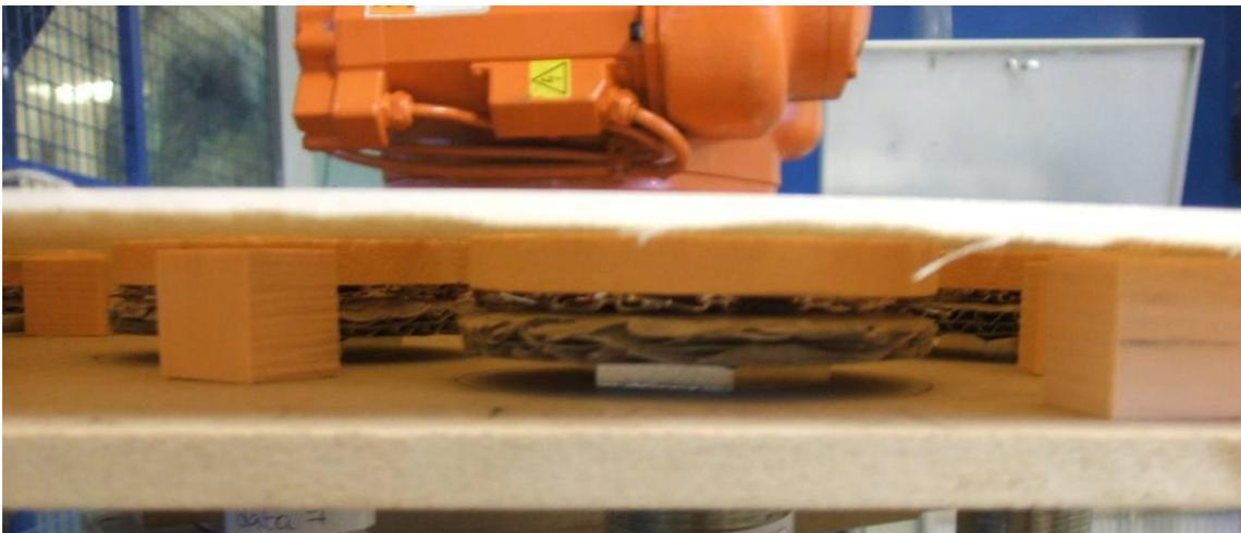
**Figure 46 Lateral board view with blocks within layers**
