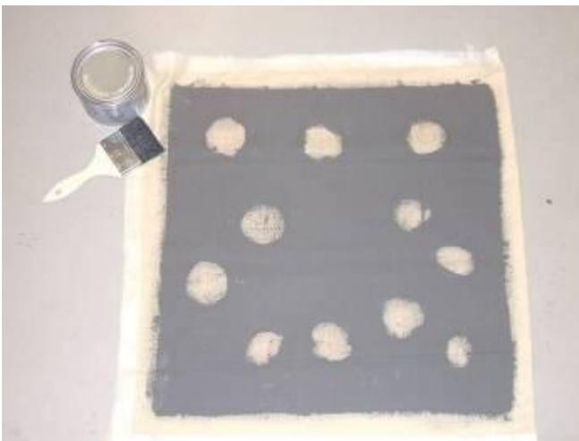
**Figure 28** Fabric painted with the metal painting for the magnet attachment
