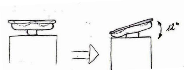
Figure 24 Sketch of the plunger movement
