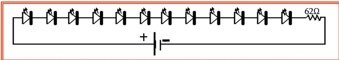
Figure 54 The blue diodes circuit
