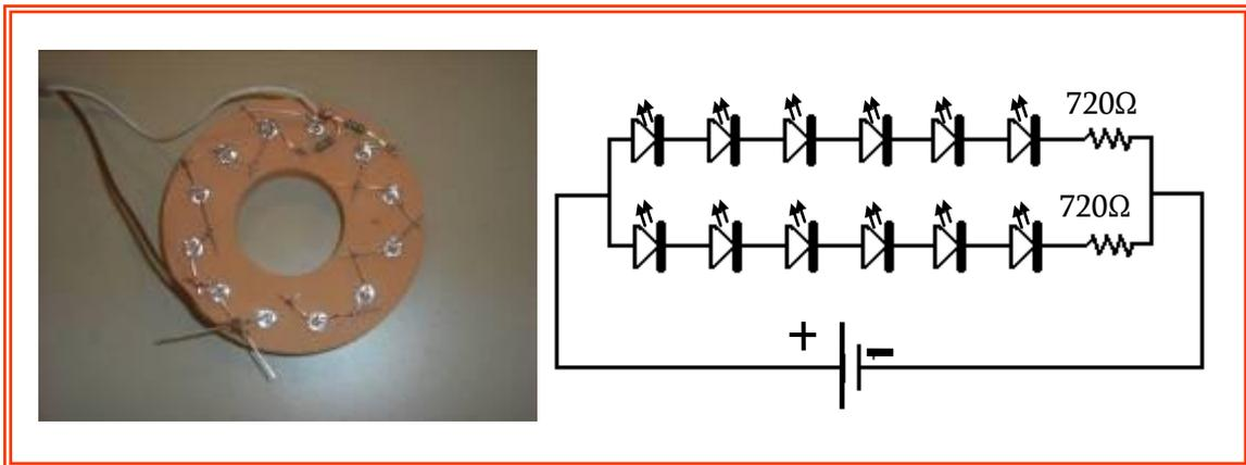
Figure 53 The blue diodes circuit
