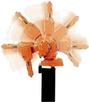
**Figure 7 Robot movement area. ABB Robotics (2009)**
