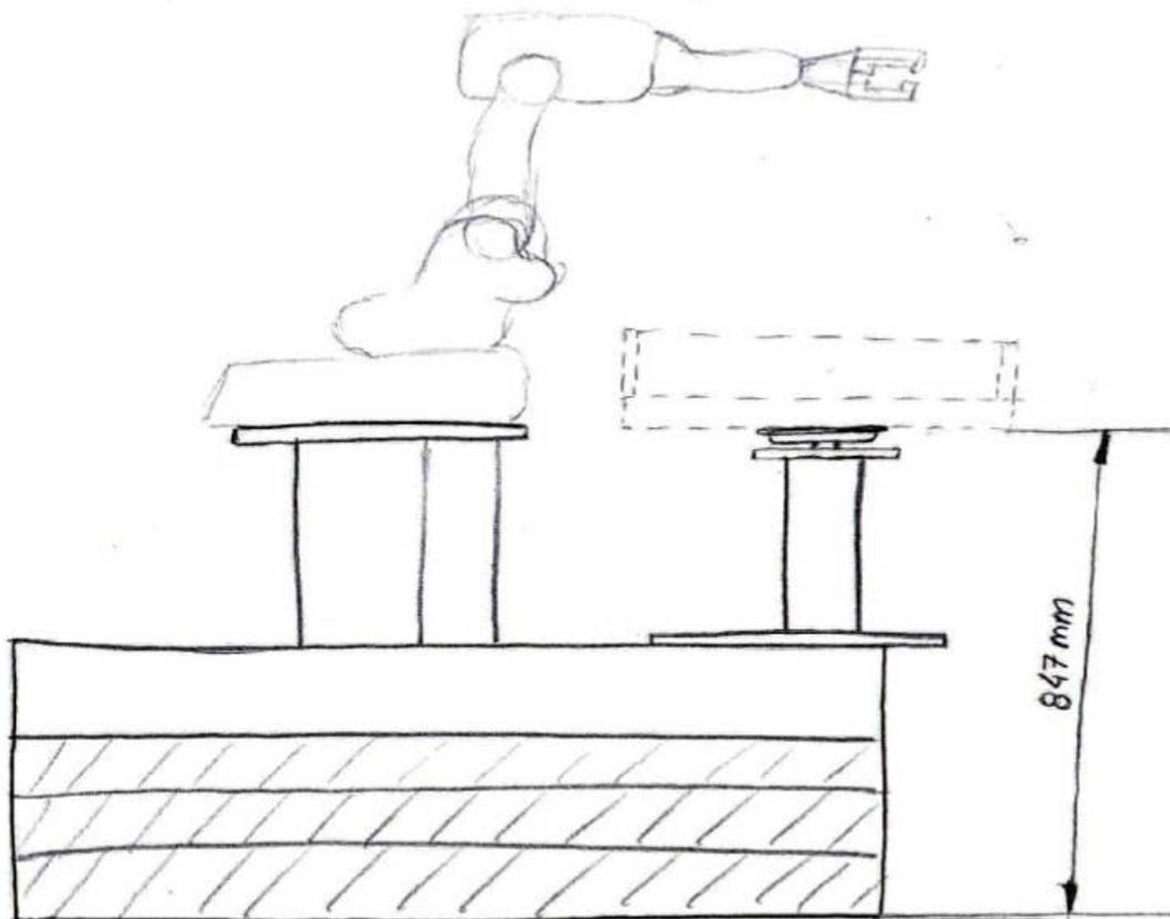
**Figure 35** Disposition of the support of the board on front of the robot.
