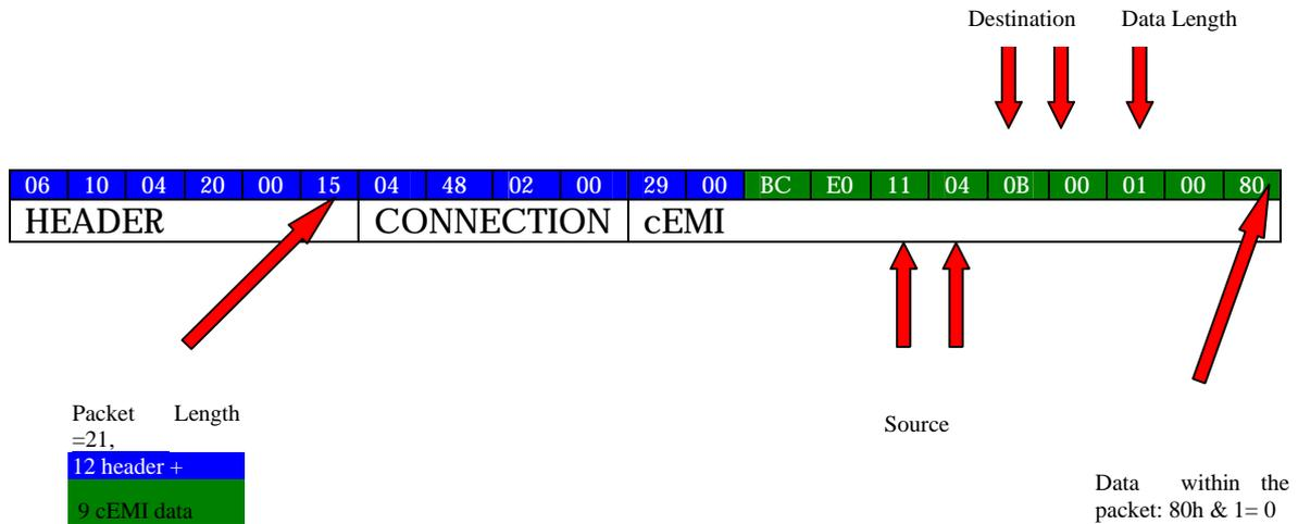
Figure 16: KNXNet/IP frame.
