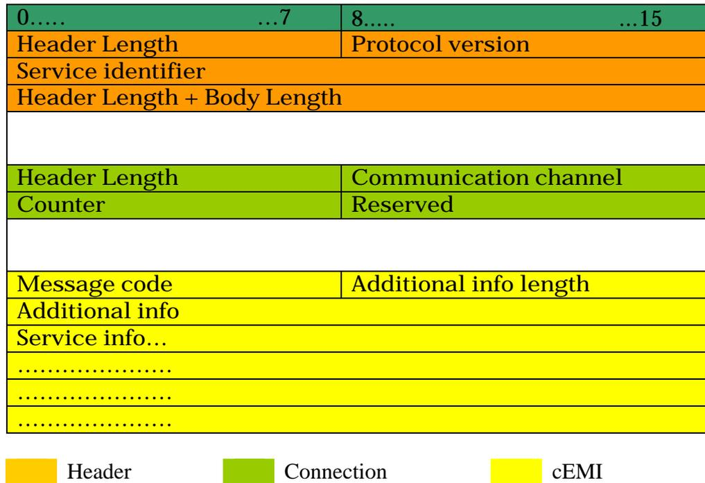
Figure 14: KNXNet/IP REQUEST frame.
