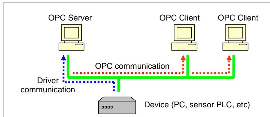
Figure 7: TCP/IP connectivity, supported by OPC standard.
