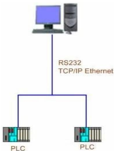
Control devices are considered hardware tools such as PLCs, which are able to gather information from industrial processes being executed in an industrial plant. They can receive information from manufacturing robot sensors, infrared cameras, temperature sensors, pressure sensors, etc.
