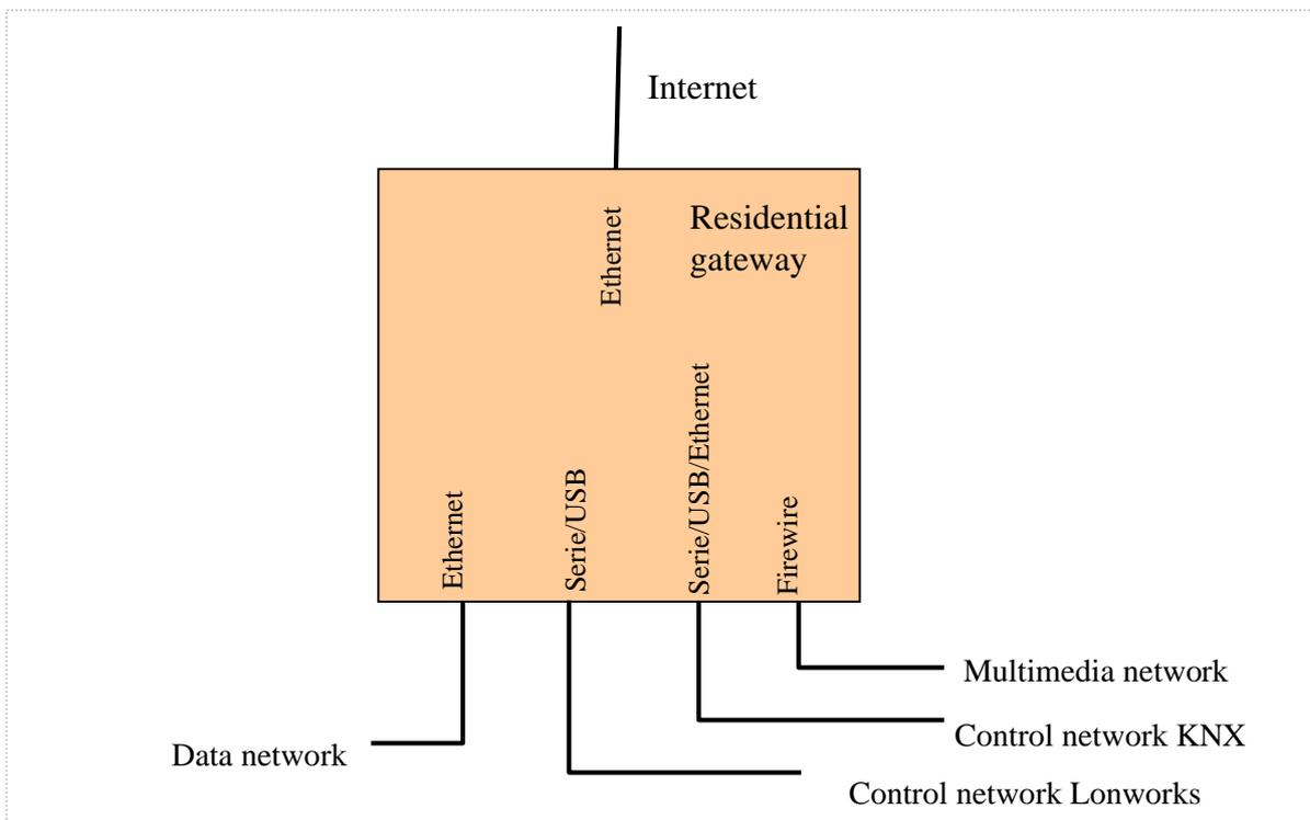
Figure 8: Basic schema of a residential gateway.
