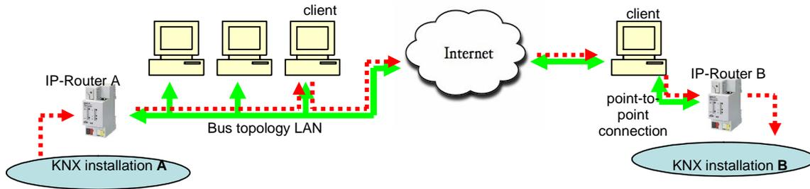
Figure 12: Schema of the model implemented by KNXNet/IP.
