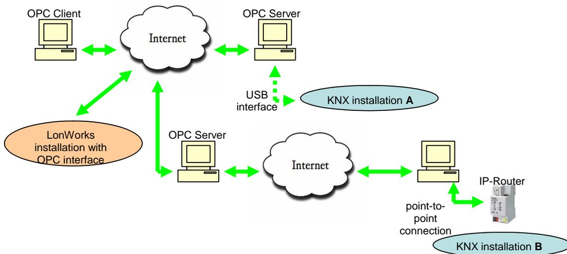
Figure 18: OPC client handling heterogeneous domotic installations.
