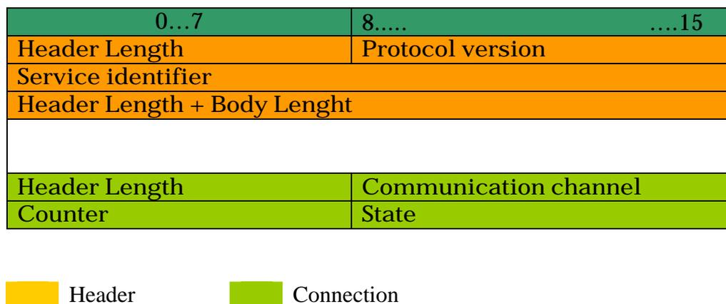
Figure 15: KNXNet/IP ACK frame.
