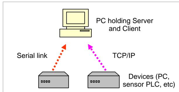
Figure 6: OPC Server and OPC Client working over the same PC.
