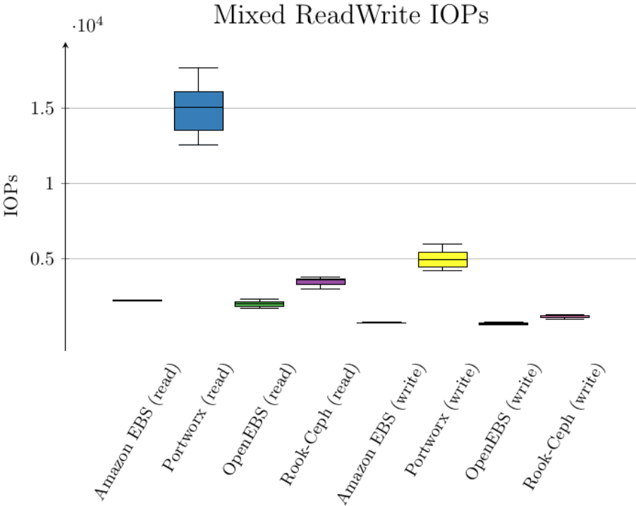
Fig 6.18. Box plot displaying the mixed read and write I/O per second on AWS.
