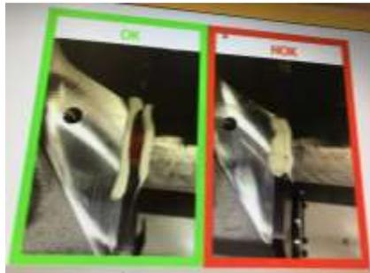
**Figure 1:** Instruction to operator for what to check for when performing the quality inspection. Correct glue strings shown to the left (OK, green box), incorrect glue strings shown to the right (NOK, red box).
