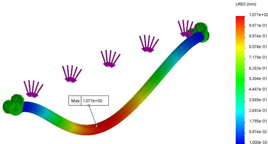
Figure 23. FEM results for  $a_1$  beam. Resultant displacement.
