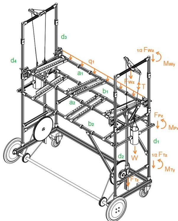
Figure 21. Nomenclature of the main forces acting on the most critical beams.
