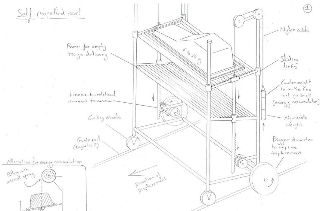
Figure 13. "Self-propelled cart". Refined concept.
