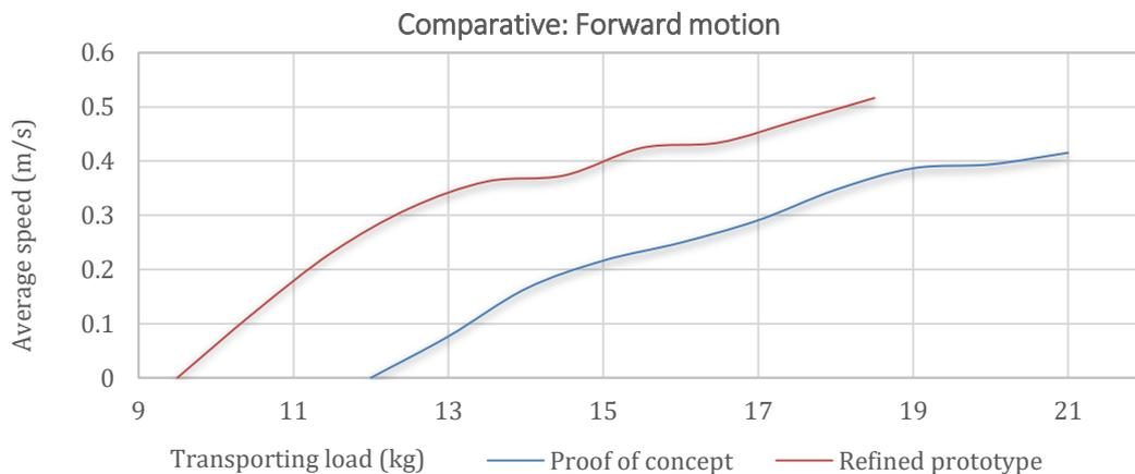
Figure 39. Comparative of the performance of prototypes.
