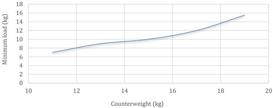
Figure 36. Values of counterweight (X axis) and minimum working load (Y axis).
