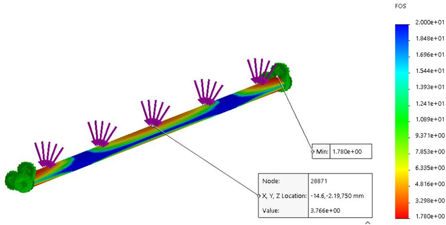
Figure 22. FEM results for  $a_1$  beam. Factor of safety.
