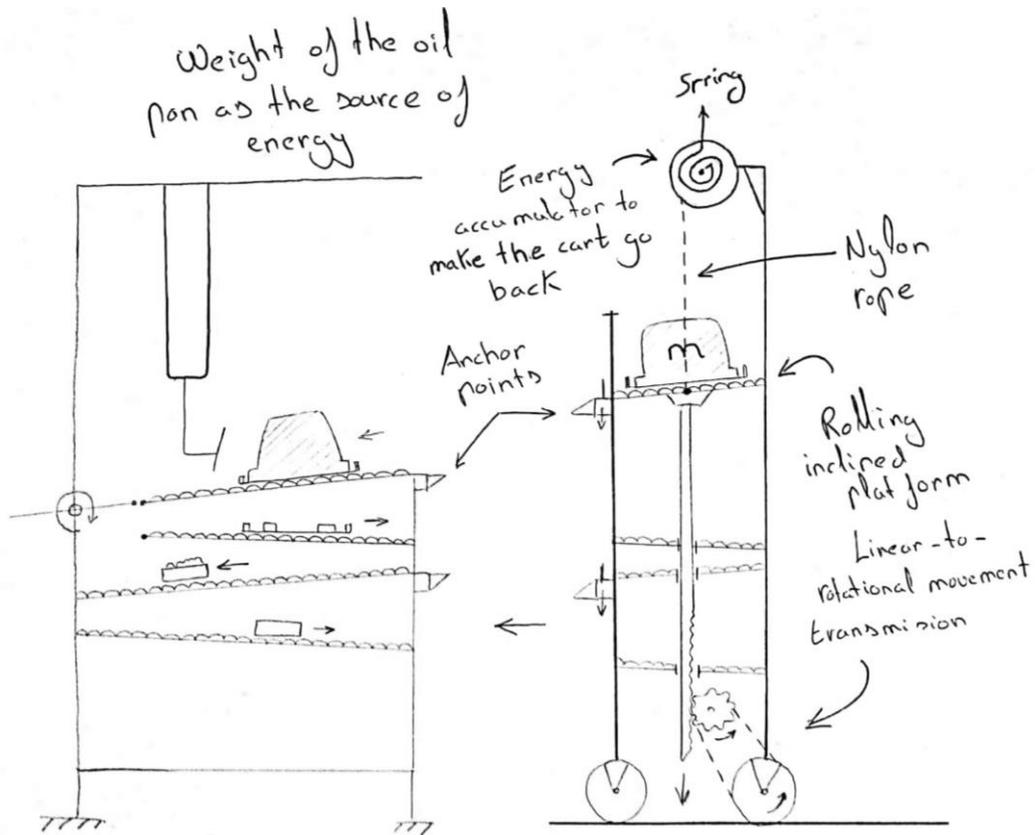
Figure 10. Sketch of the "Self-propelled cart" concept.
