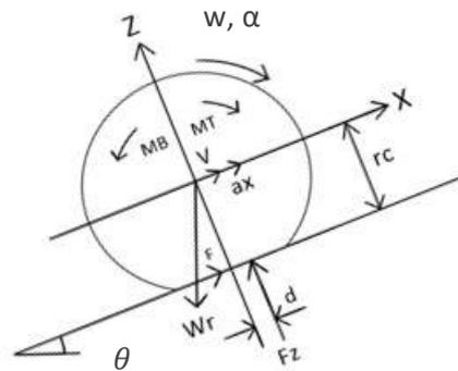
Figure 20. Sketch of the forces and moments involved in a vehicle's wheel.
