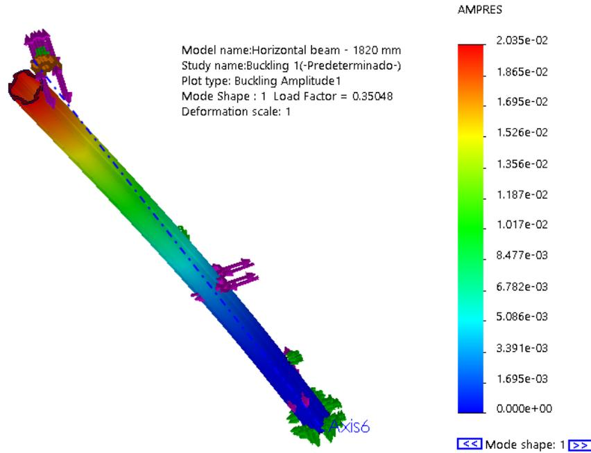
Figure 24. FEM results for  $d_1$  pillar. Buckling effect.
