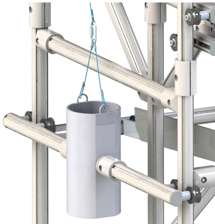
Figure 17. Detail 2. Constructive solution for adjustable counterweight.
