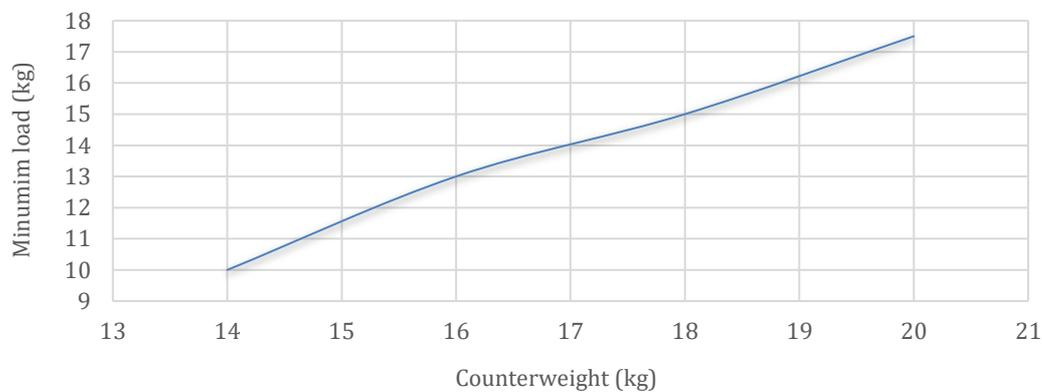
Figure 31. Values of counterweight (X axis) and minimum working load (Y axis).
