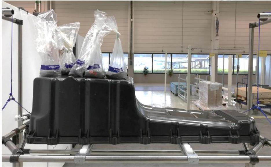
Figure 30. Use of metallic sandbags for varying and measuring working loads.
