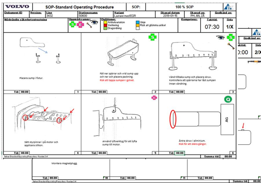
Figure 40. SOP layout example.
