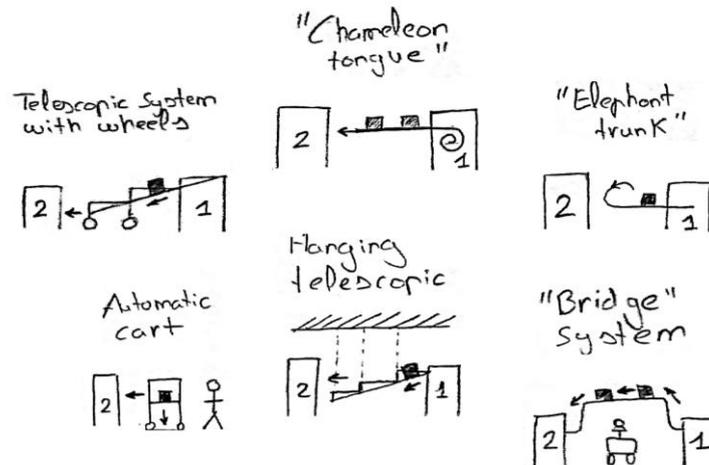
Figure 7. Scheme of the ideas generated through brainstorming for the transport function.
