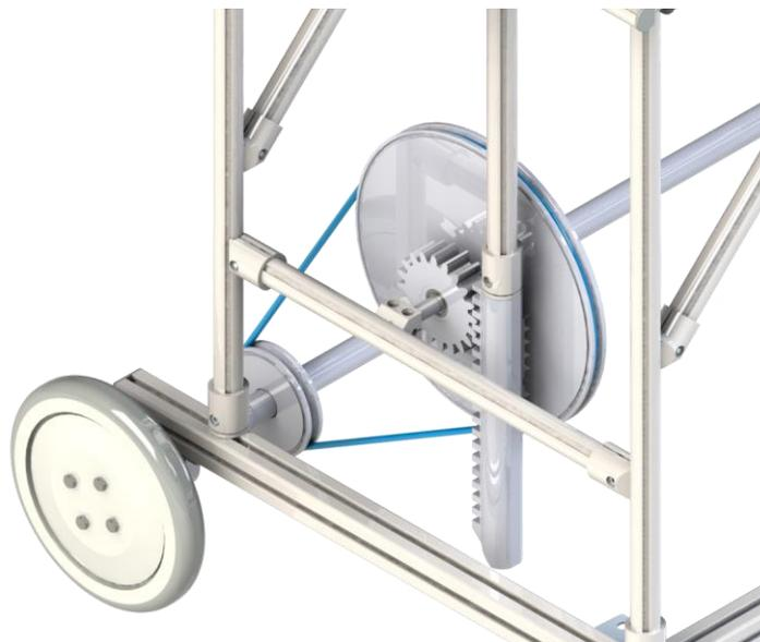
Figure 19. Detail 4. Constructive solution for the transmission system.
