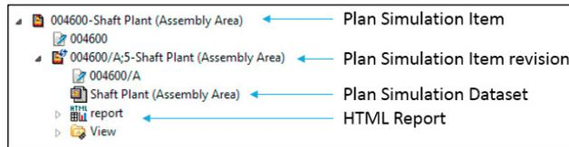
Fig. 5. Plant Simulation Item and its attachments
