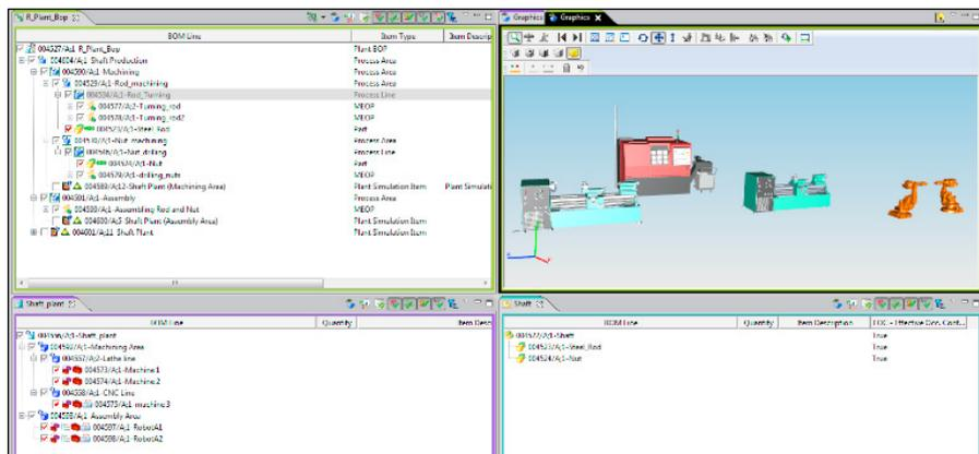
Fig. 3. BoM, BoP, BoR with 3D models of resources in Teamcenter
