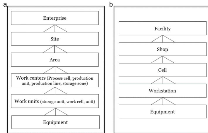
Fig. 1. Manufacturing system Models (a) IEC 62264-3; (b) NIST
