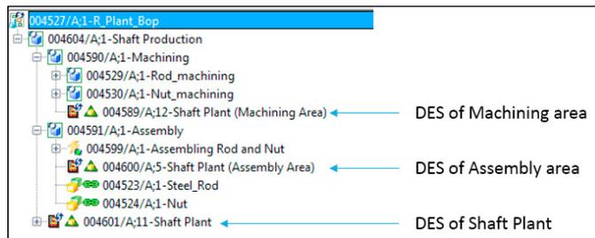
Fig. 7. Bill of Process for Shaft Manufacturing
