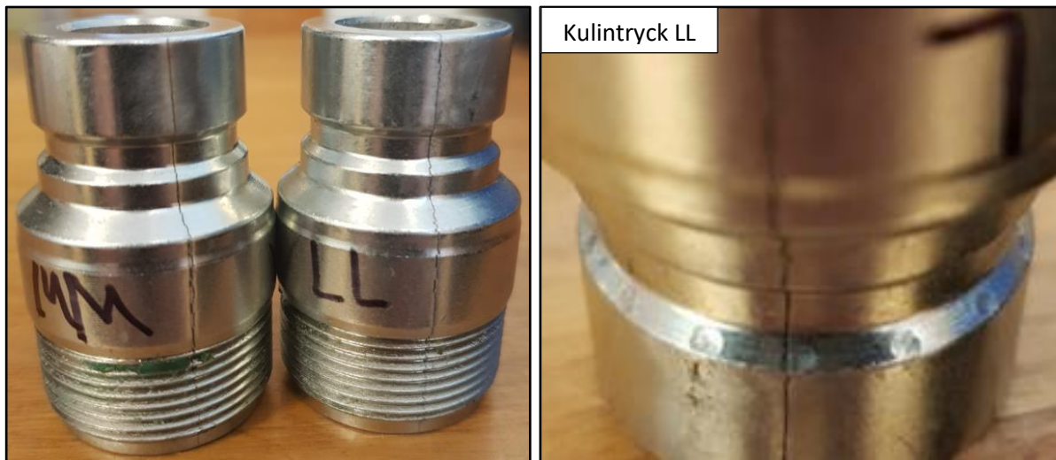
Figur 3.2.4. Spricka i hanes nippelhus, test MM & LL.
