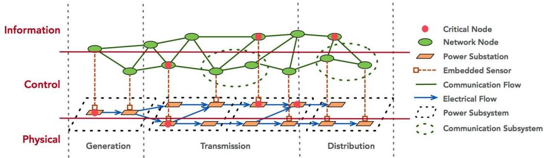
Figure-1. Multidimensional network illustration in smart power-grid structure
