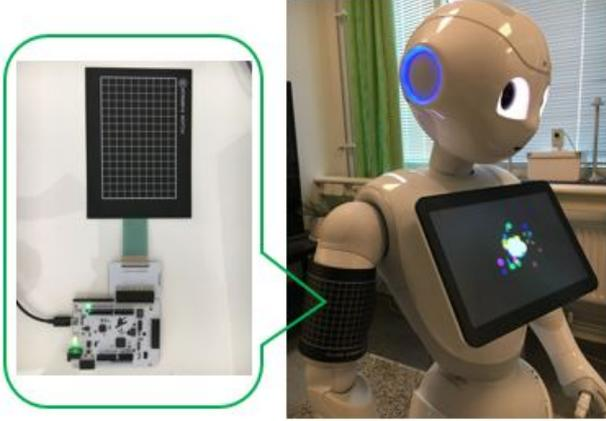
Fig. 1 Left: The Kitronix matrix array sensor and the Snowboard microcontroller. Right: the sensor is placed on Pepper's arm.
