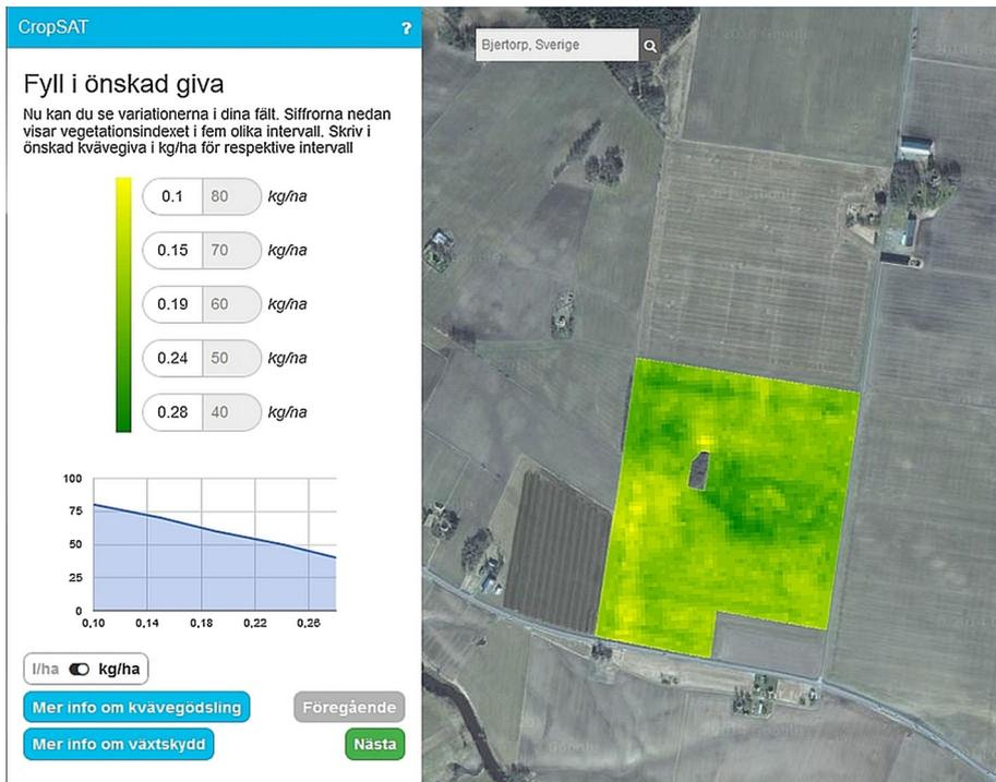
**Fig. 1** Variation in vegetation index calculated by the AgriDSS CropSAT (<http://www.cropsat.se>) from a satellite image and visualized on a chosen field in Google Earth. Five levels of nitrogen application are set and can be used as a basis for calculations of a VRA
