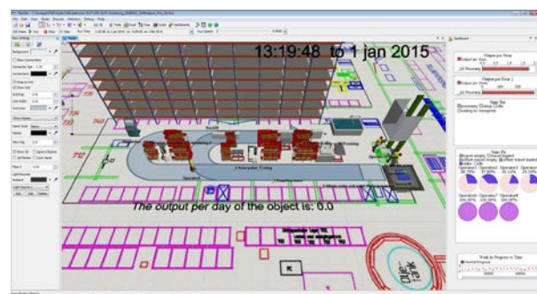
Fig.3: Simulation model of a manual production line
